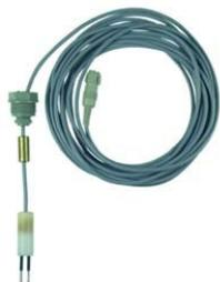
The supplied conductivity Level Probe is used as a minimum water level detector in the rainwater tank. The standard length of cable supplied is 15m. This can be extended to order, up to 100m. It carries a very low voltage/current.
